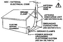
INSURE SAFE ANTENNA AND CABLE CONNECTIONS If an outside antenna or cable system is connected to the equipment, be sure the ANTENNA equipment, be sure the DISCHARGE UNIT antenna or cable system is (NEC SECTION 810-20) grounded so as to provide some protection against built up static charges and voltage surges. Part 1 of the Canadian Electrical Code, in USA Section 810 of the National Electrical Code, ANSI/NFPA
