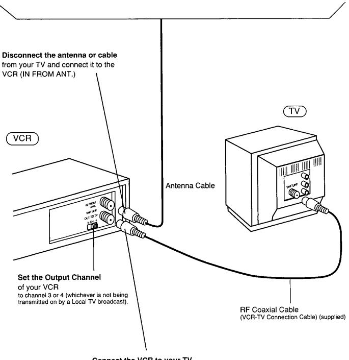
Connect the VCR to your TV with the RF Coaxial Cable (OUT TO TV).
